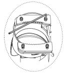
Mark:If the machine cannot pull down the shuttles, please adjust the metal clamp.
