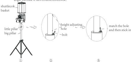
2. You can adjust the height location hole when you need to adjust the height of ball shooting, holding the turb by hand (Be sure to make the hand position within the yellow warning line, otherwise may lead to accidents), reach the height you need, aim at the location hole and fasten.
