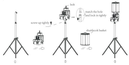
Please follow the 1, 2, 3 step above and install the main machine, please note lock the screw when install the main machine as picture 3.
