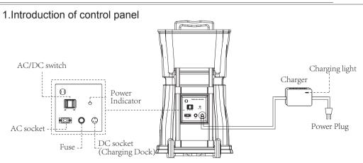
( Note: The charger is only used for charging, Don't use it as the power cord ) ( Red light means charging.Green light means full charge. )
