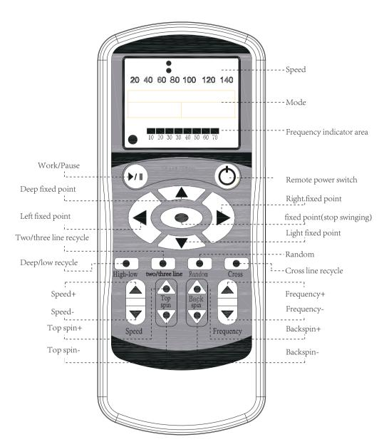
Note: Push and hold the ON/OFF button for 3 seconds to turn the remote control on.
